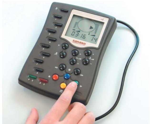
The delegate's STS position is equipped with a Lab 100 User Audio Panel, headphone connectors, a gooseneck microphone and an illuminated switch for activating and muting the microphone.
